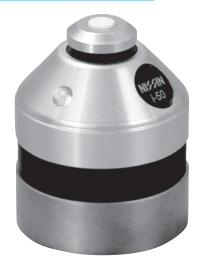
Tool Setter-i has been developed for ultra-highspeed spindle with the machine tools (10000rpm). It is available to measure plastic, wood and some other materials which block electricity. Magnets are attached at the bottom, so it can be used with both vertical and holizontal machining tools.
