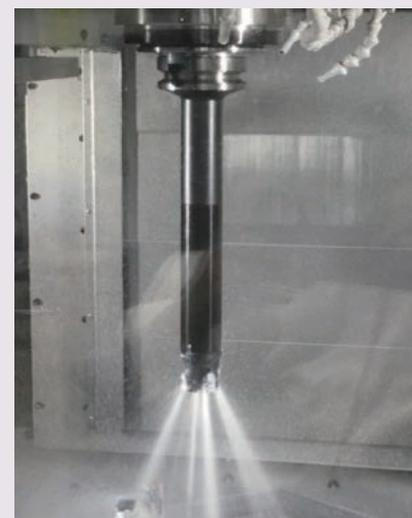
This product combines our damper technology, which boasts many achievements and increases the damping effect and reliably damps chatter. Achieve stable processing! Resolve the reduction of surface roughness, defective processing dimensions, and shortened cutting tool life at once!
